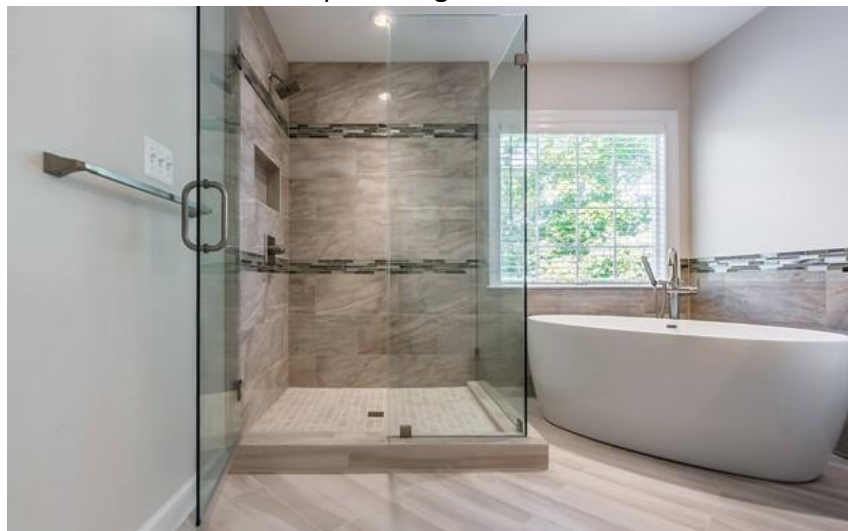
Figure 1: Example of frameless shower enclosure with stationary and operating panels
